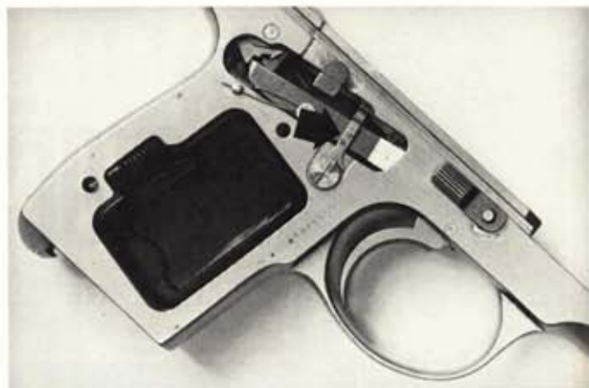
Budischowsky safety is spring finger held by large head screw beneath grip panel above magazine well.
