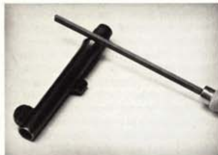
This S&W 1917 barrel required use of a file on shoulder before it would turn up far enough.
