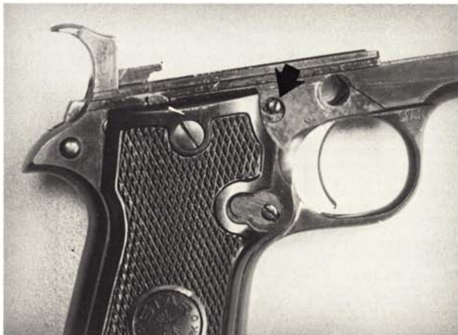
Star SM auto pistol in .380 has magazine safety as a plunger in frame at upper front corner of right grip; remove by rotating slotted head.
