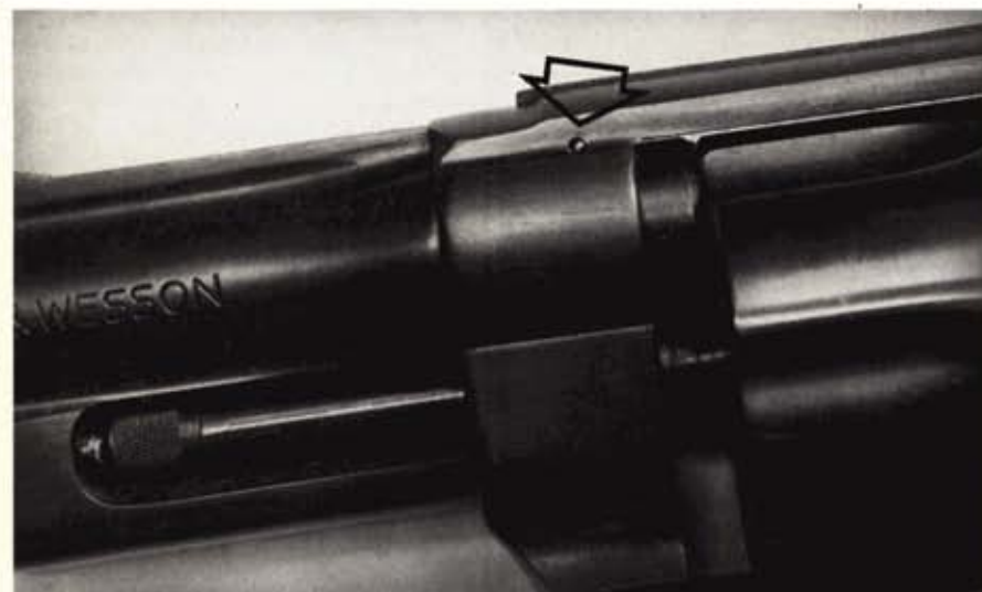
Before even thinking about removing a barrel, always examine the frame for any pins or retaining devices; this S&W barrel is held by a pin.
