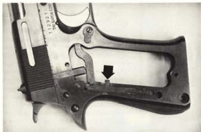
In big frame Star auto pistols, the magazine safety is the vertical leaf spring in frame behind magazine.
