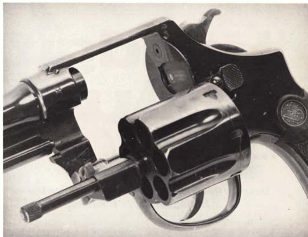
With cylinder open, the third lock—plunger on bottom of ejector rod shroud—is readily apparent. Note British proofs at top of frame.
