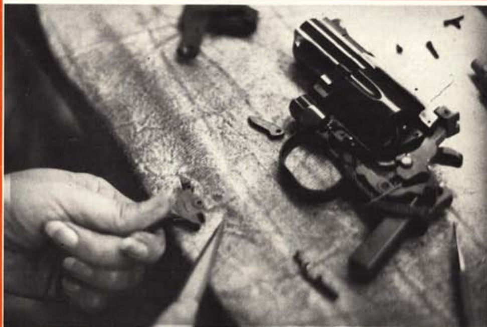
For a slicker action, author recommends nothing more than a little honing and application of molybdenum disulphide between the parts.
