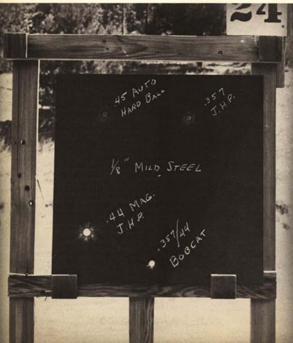
Steel plate shot at 50 feet. Only the .44 Magnum and the Bobcat penetrated the plate.
