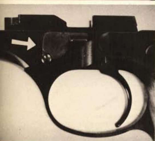
Take-down latch of the Model 92 shown in open and closed position. Lock button is pushed from the right side of frame to unlock.
