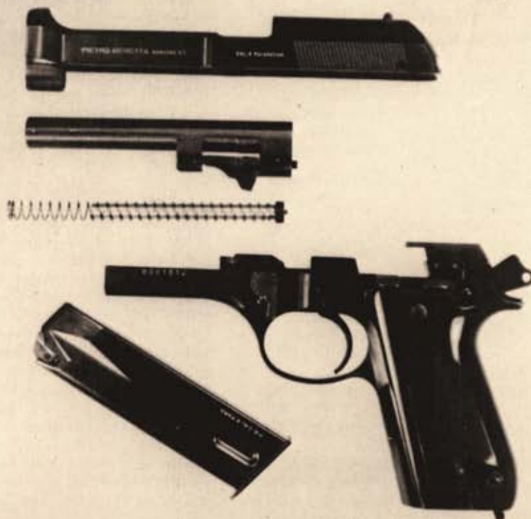
The Model 92 field strips down to five major components.
