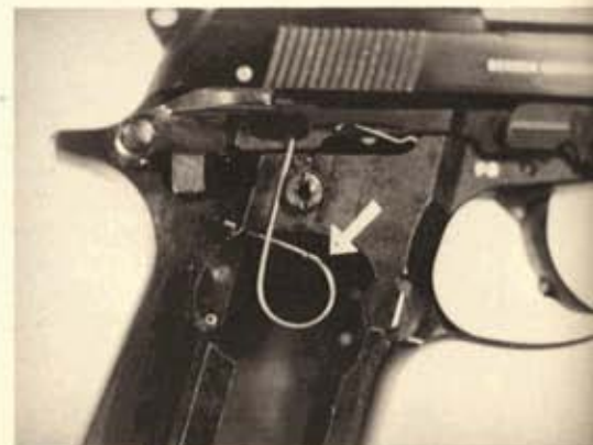
Model 84 magazine safety exposed with grip panel removed. It can be easily removed without tools.
