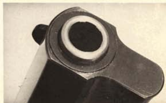
Close fit at breech and muzzle ends of slide result in a tune-up that rivals a full accuracy job.
