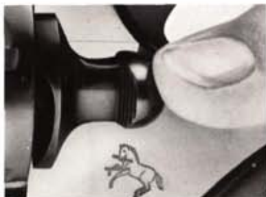
Thumb latch pulls toward rear on a Colt, precluding accidental cylinder release.
