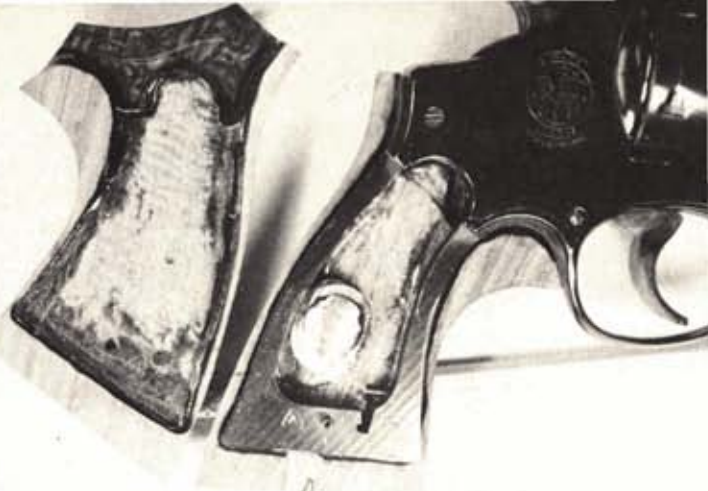
Ready for final fitting, the assembled halves are snapped together and epoxy has been liberally applied to the grip panel for final bond.
