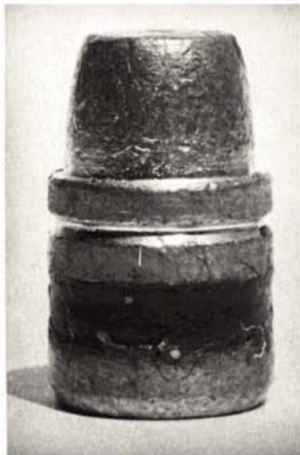
This H&G bevel base semi-wadcutter shoots consistently well in nearly all .44 sixguns. Cast hard, sized .001 over groove diameter and properly lubed, this one is a winner.
