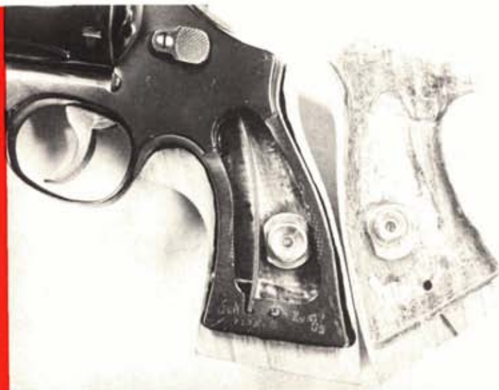
An inside look at the finished product: screwless grips that are both secure and functional. Note close fitting, but not tight, inletting.
