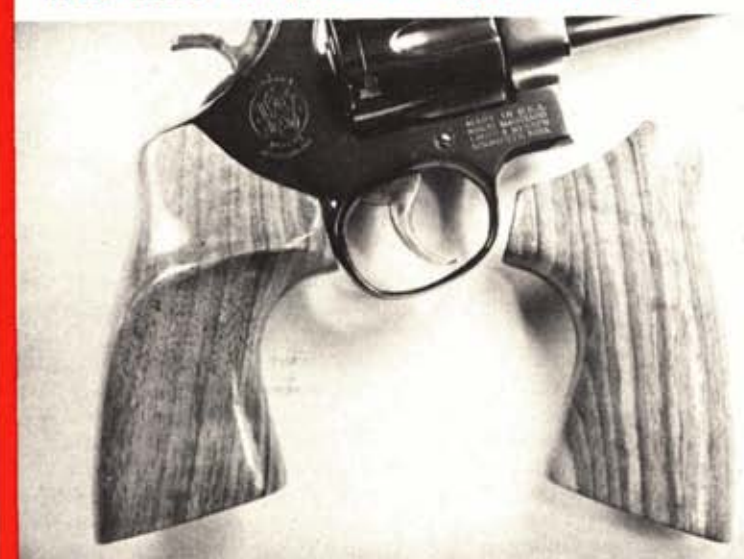
Seen from the outside, the finished grips are coated with a sweat-proof 2-part epoxy varnish. The handfitting contour allows a firm hold.
