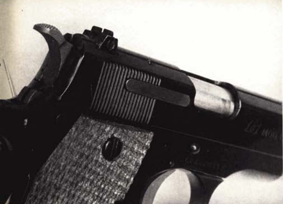
Adjustable for windage only, the Model D's rear sight unit is of the traditional patridge configuration and is not shadow-boxed. Opposing screws must be loosened and tightened to move the sight leaf laterally. Though simple in concept, the arrangement works remarkably well.
