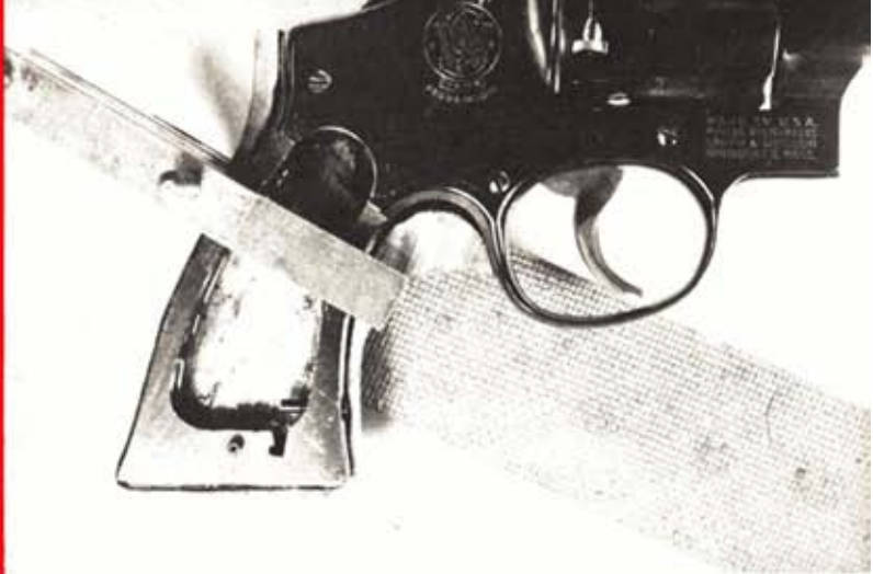
The loose inletting is tightened by epoxy bedding to form a secure, split-proof fit on the hard-kicking Model 29 .44 magnum.
