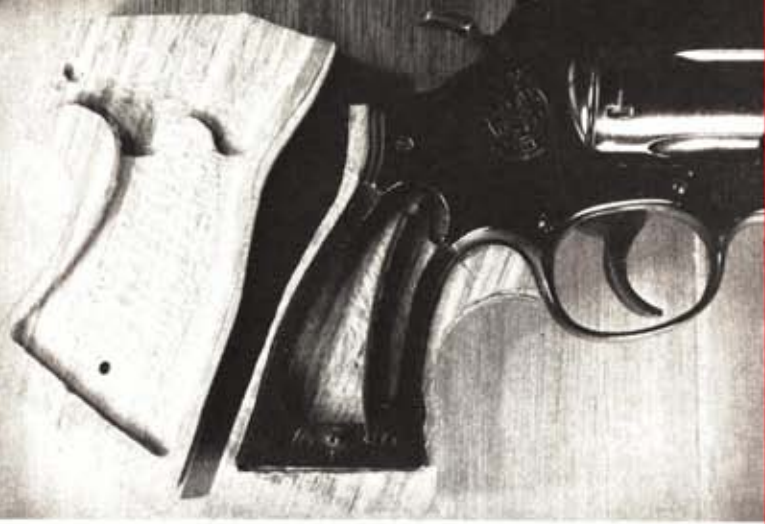
Roughly inletted grips for a Smith & Wesson M-29 have been shaped with a router bit on an electric drill press prior to fitting.
