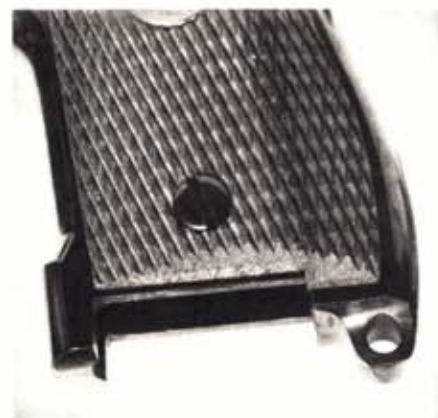
The Model D's grip frame is relieved to allow the grooved finger slots of the magazine to be easily gripped during reloading.
