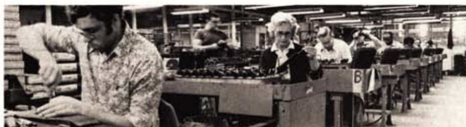
Hand honing and fitting give a Colt revolver its characteristic velvet smooth action.
