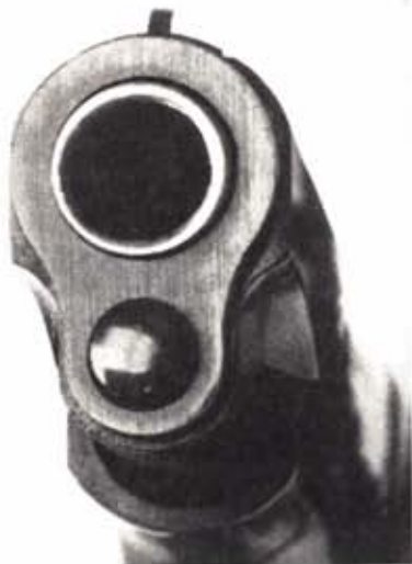
A muzzle-on view of the Model D shows the little .380's obvious Colt influence. The recoil spring guide can be seen protruding from the muzzle's front bushing.
