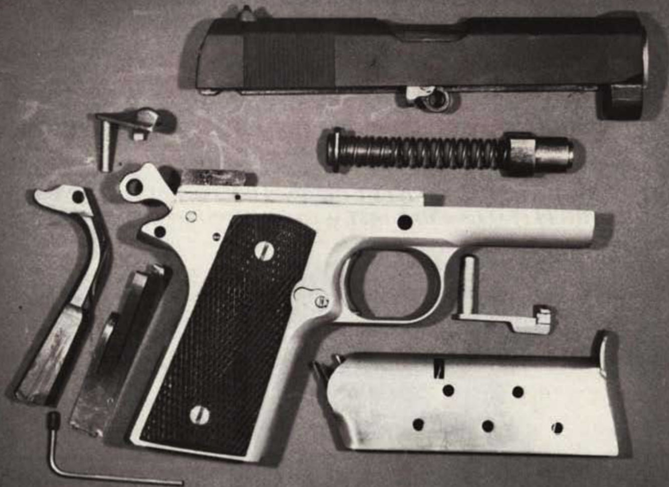
The shorty .45 is shown duty-stripped. Fourteen components were modified.
