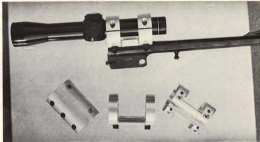
Three experimental mounts are shown beneath the final version which is mounted atop a specially machined Thompson/Center Contender tube.
