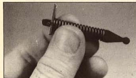
When spring and plate are captured by takedown pin — spring assembly can be used for further takedown operations.
