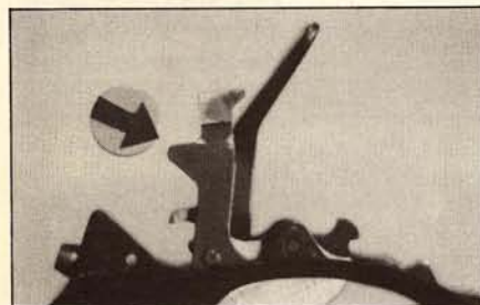
Arrow shows lobe on back of hand. This is critical during reassembly.
