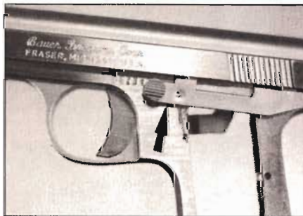
The manual safety level (arrow) is its own positioning spring, but it is not flexed enough in normal operation to make breakage likely.
