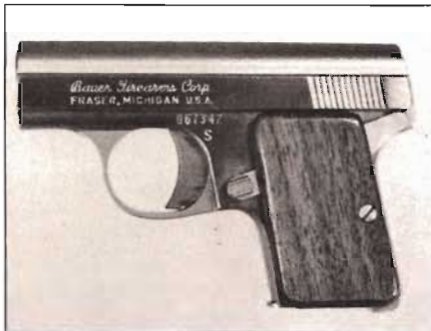
The Bauer Stainless Steel .25 automatic. The one shown is the author's own gun, and has been modified by removal of the sights and thinning of the grips.
