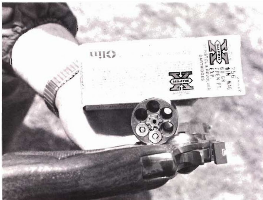
Specially-reamed cylinder is evident in this shot. Backouts did occur with some handloads but factory fodder worked well.
