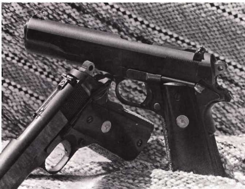
K-Sights on the "workhorse" Colt gives a lower sight plane, and, of course, puts finely adjustable sights where once stood only the "windage only" plain combat sight.
