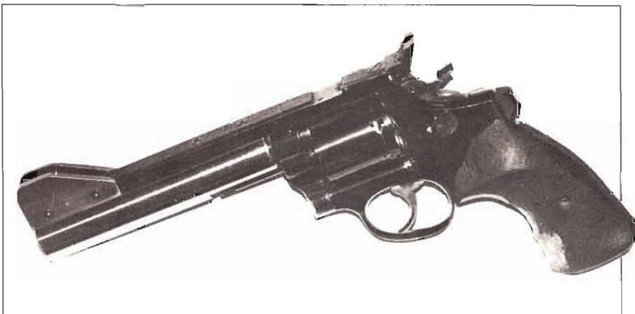
Here's Reed Knight's (1306 29th, Vero Beach, FL 32960) conversion of the Model 53 Smith and Wesson Jet to .32 caliber.
