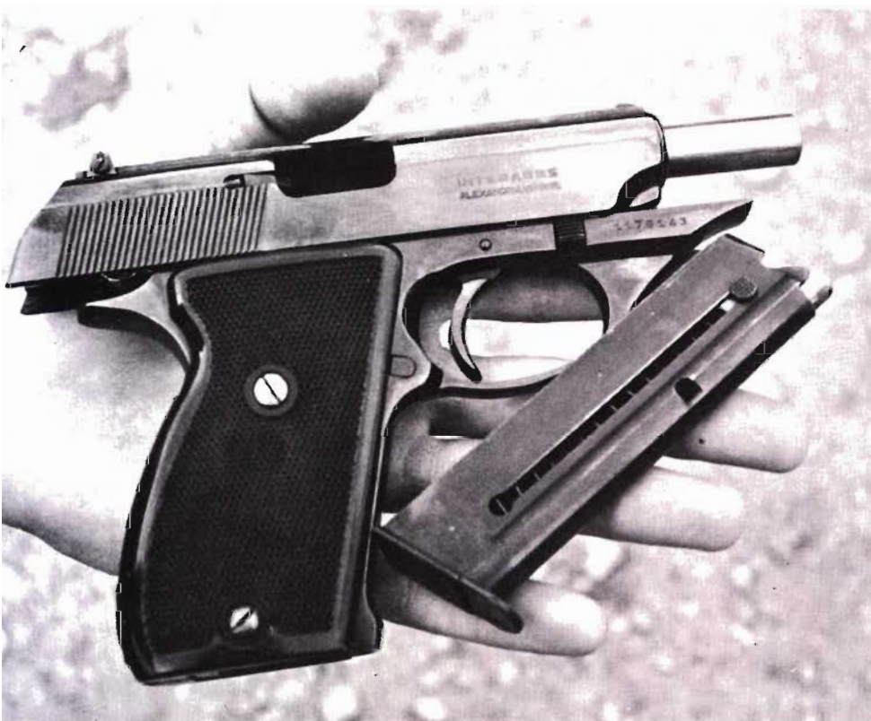
Above: The Astra is small enough to fit in the palm of your hand, making it an easily concealable back-up piece. Right: Takedown is easy and takes only a few seconds. Takedown release is located just forward of the trigger, and projects on both sides of the frame.
