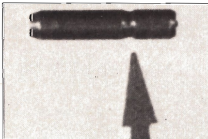
A spring in the left side of the breech block locks into a groove (arrow) in the retaining cross-pin to hold it in place. When replacing pin, the groove must go to the left side.
