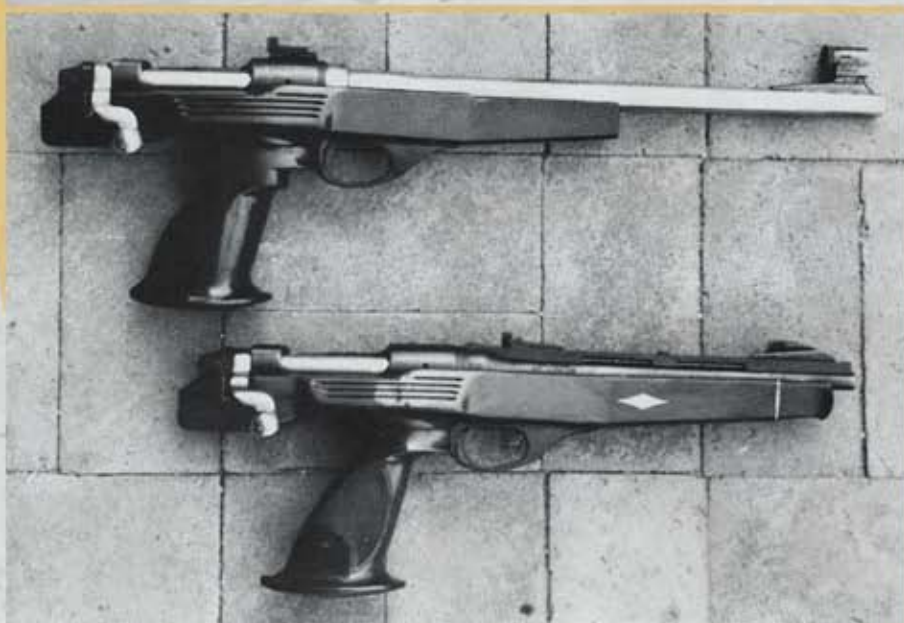
Top: Here's the improved, altered grip—in the raw, so to speak. But this is a step towards a lot less recoil pain. Middle: Here's the basic package. It includes the barrel, dies, gauges and, of course, the stock. Bottom: Before and after. The modification to the factory stock's forend to accept the larger barrel can be seen through comparison.
