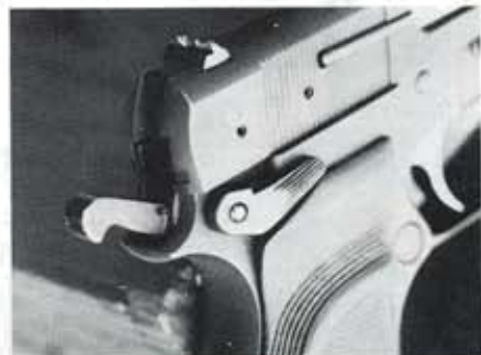
Note here the safety pin at base of hammer. Note also the clean design of the Southside thumb-safety lever.
