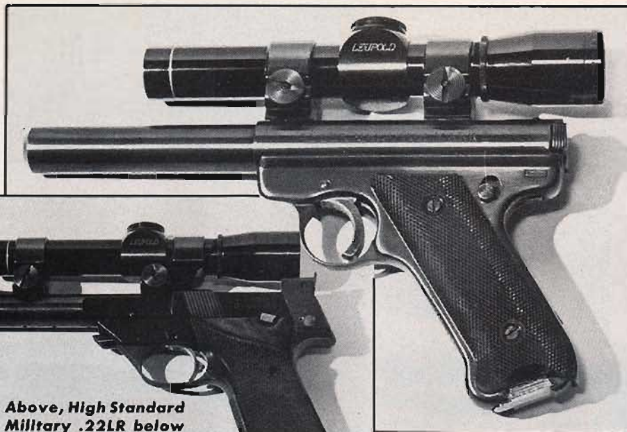
Above, Ruger Mark I with bull barrel sporting Leupold Model 8 2X mounted with Weaver 1" rings and Weaver No. 32 bases.
