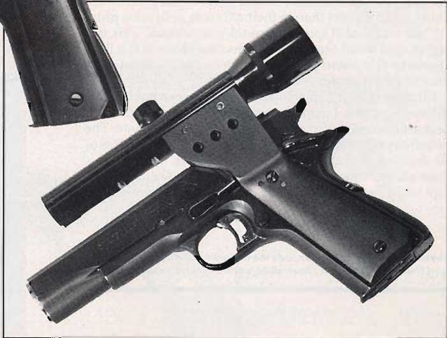
Colt National Match .38 Special midrange with Bushnell Magnum Phantom 1.3X mounted on a Custom Grip Plate Mount by D. W. James solves problem of the slide with scope and mount attached that becomes too heavy to function right.
