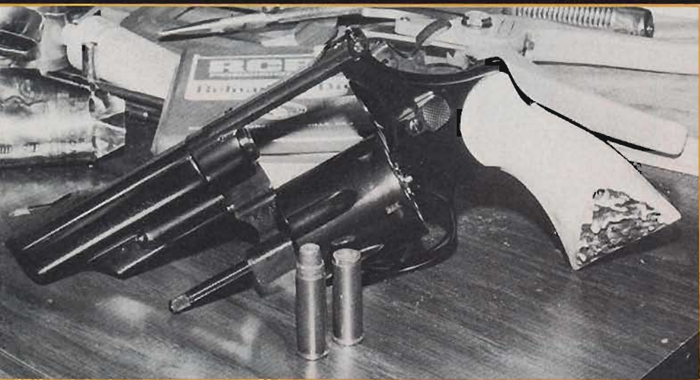
Above, S&W Model 57 .41 magnum revolver is in the "heavy" caliber category and in the tests showed the slowest rate of recoil recovery of all four guns.
