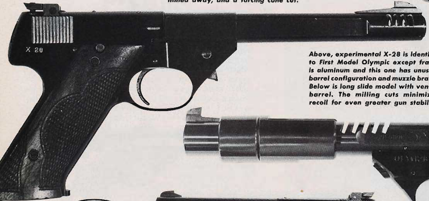
Above, short slide identical to pistol used by Col. W. W. McMillan when he achieved Gold Medal for U.S. in 1960. Left, the only remaining example of a "jump" barrel. Entire bore has been milled away, and a forcing cone cut.
