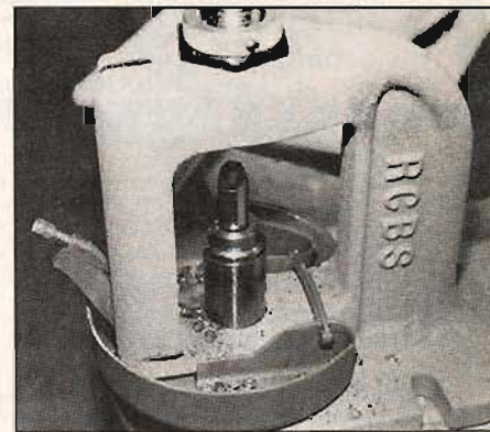
The bullet just seated, a .45 cart-ridge, is withdrawn from the press.
