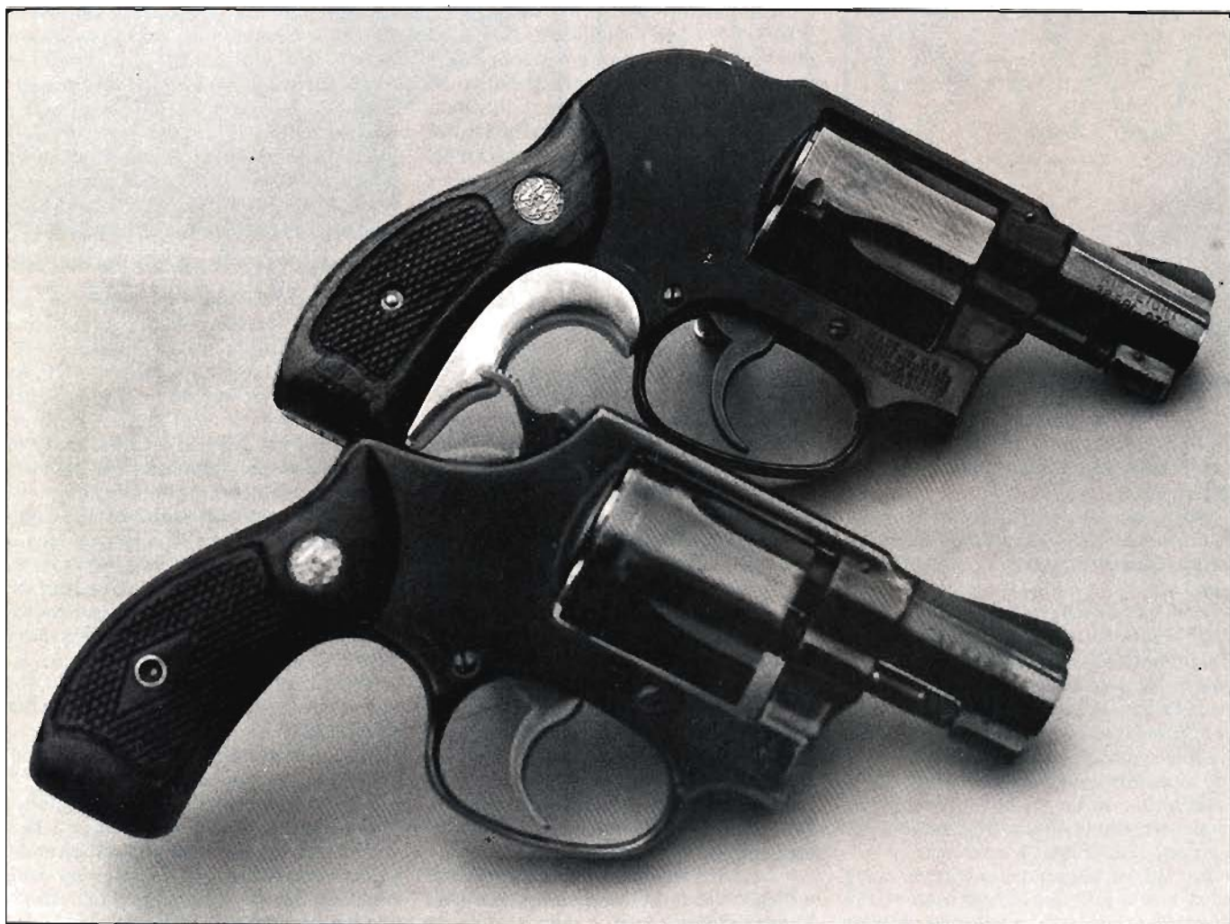
Top of page: Colt Police Positive was one of the better revolvers to be chambered for the .38 S&W. Note shorter cylinder of .38 S&W Terrier, below, compared with the .38 Special cylinder of the early Bodyguard/Airweight, top.
