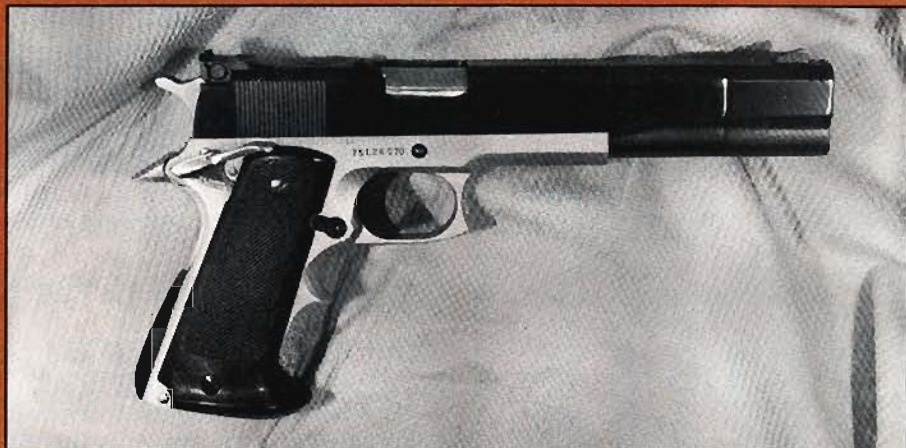
Ready to go for fast shooting on combat and bowling pin targets. The Behlert "pin gun" system costs about $450, reduces recoil and increases sight radius.
