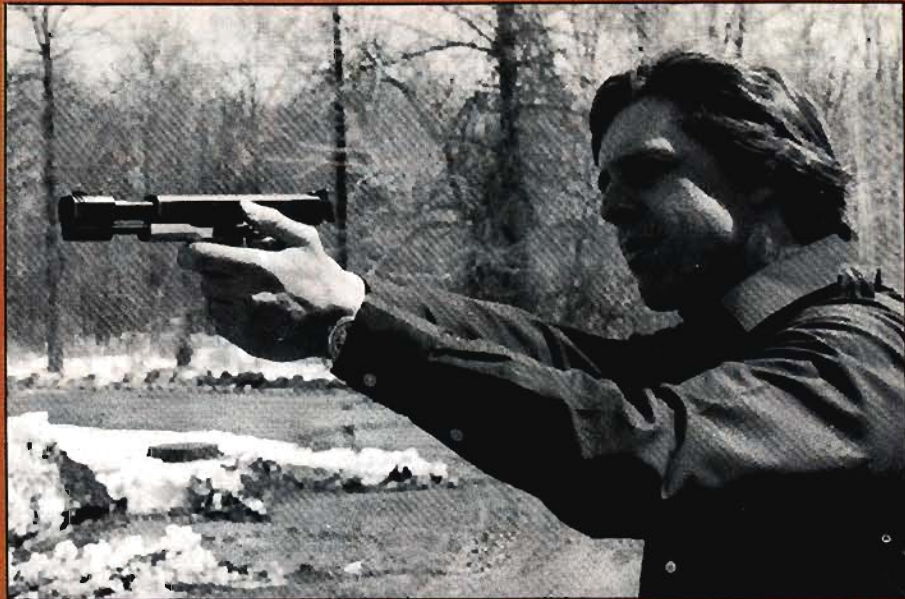
Behlert catches a sight picture with his .45 "pin gun." Note the extra heavy, vented barrel extension. This is what keeps muzzle on target with full loads.
