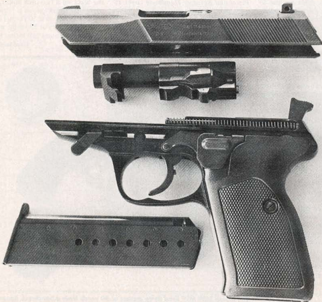
Field-stripping the Walther P5 takes only a few seconds.
