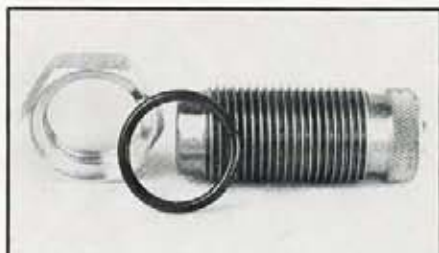
The expander/flaring die is adjusted by raising or lowering the lock rings.
