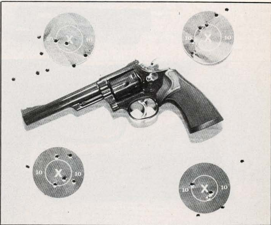
The 6-inch S&W M19 fired three groups at 50 yards from a benchrest. Speer 125-grain JHPs were used. After sight corrections between strings, and disregarding called fliers, this .357 Magnum is capable of firing 3-inch groups at 50 yards.
