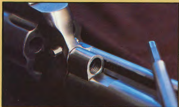
Interrupted threads of barrel, and cylinder locking device are shown in photos at left. Interchanging both cylinders and barrels is easy task.
