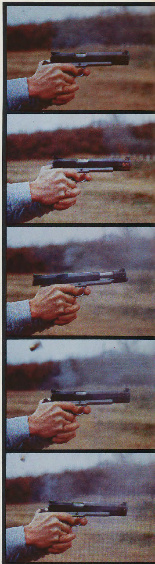
Photo sequence (top to bottom) is graphic demonstration of effect of Abater recoil device on Gammon II.
