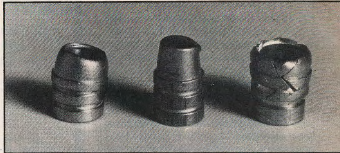
A demonstration of comparative hardness by nose-to-nose crushing of (L to R) wheel weight, heat-treated, and linotype. The heat treated bullet easily punches well into the nose of the others.
