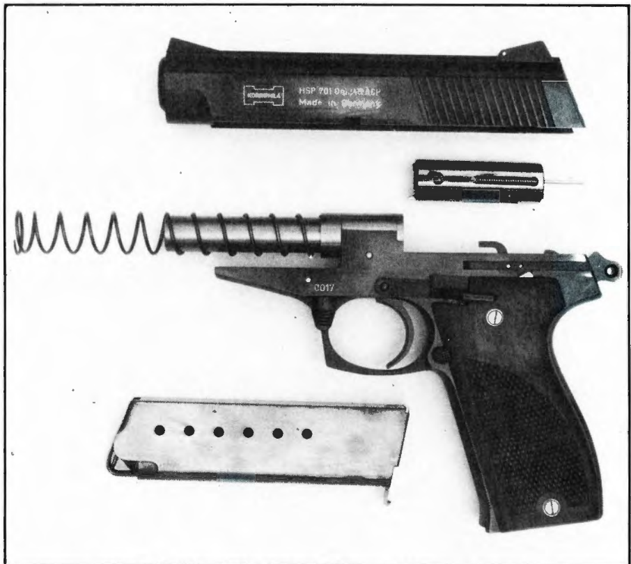
The German auto field strips into four parts. A simple and reliable design.
