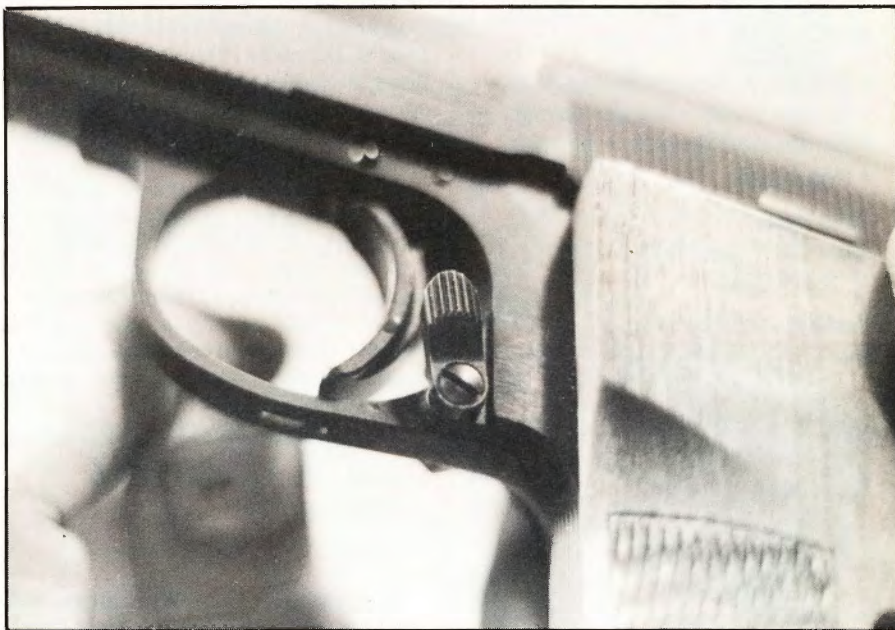
The optional manual safety is shown in its vertical "off-safe" position.
