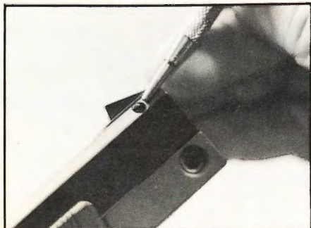
Small screws on base of front sight offer windage adjustment to blade.
