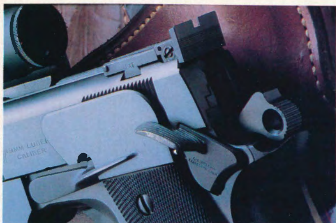
Slide shield prevents thumb from rubbing slide.
