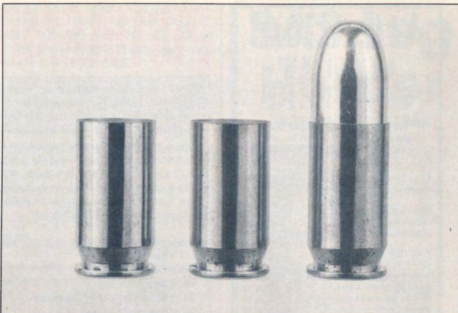
Left to right: primed case; flared case; flared case with bullet.
