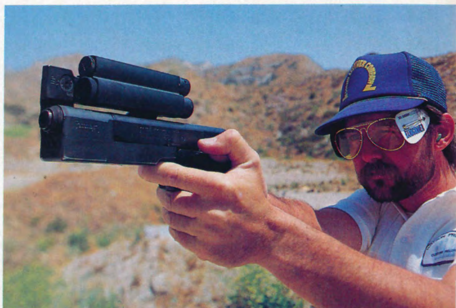
Pachmayr's Paul Liebenberg (above) test fires a modular pistol. Note elevation adjustment (above and left) for Aimpoint sight.
