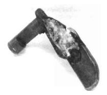
some pressure must be applied to hold the extension snugly against the safety. Their irregular shapes preclude the use of the usual clamps, so position the safety in a vise or some sort of holding fixture (visegrip pliers will do) and then bend about 2 inches of the end of an 18-inch rod or strip of some metal as shown and file the end to a point. Attach a crossbar of some sort or a large C-clamp to the unbent end of the rod to give it more weight and to hold it upright.
