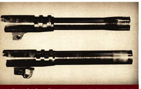
Original Colt Super .38 barrel (shown at top) had to be replaced with the Bar-Sto stainless steel barrel (bottom). Note the massive Broadfoot link. The inside of frame must be cut away to accommodate this linkage.
