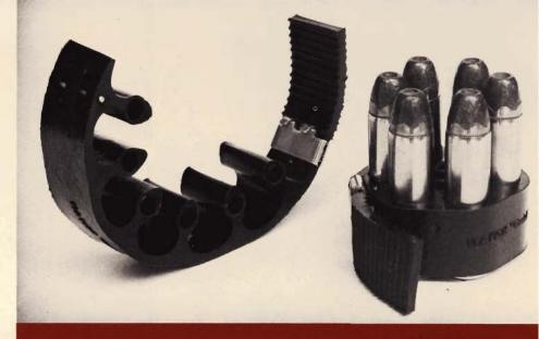
The Matich Quick Loader is unique in construction and function. The metal frog fingers engage a cross-pin to form a single strip into a circular receptacle. Pulling the serrated tab unwinds the strip and releases individual cartridges into the cylinder chambers by gravity.
