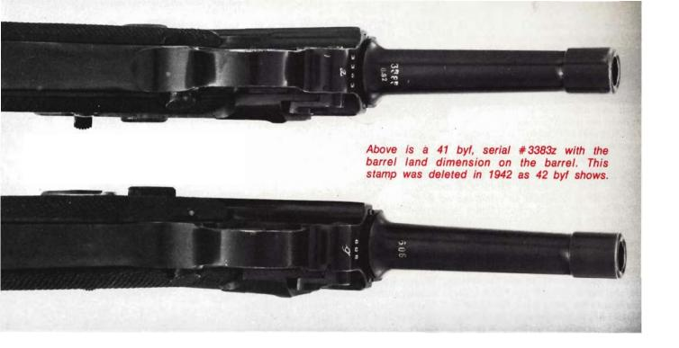
ters, the magazines were changed from nickel-plated to blued stamped steel. At this same time, Mauser stopped polishing the interior of the receiver times, although they continued to polish the frame interior horizontal surfaces until 1937.
