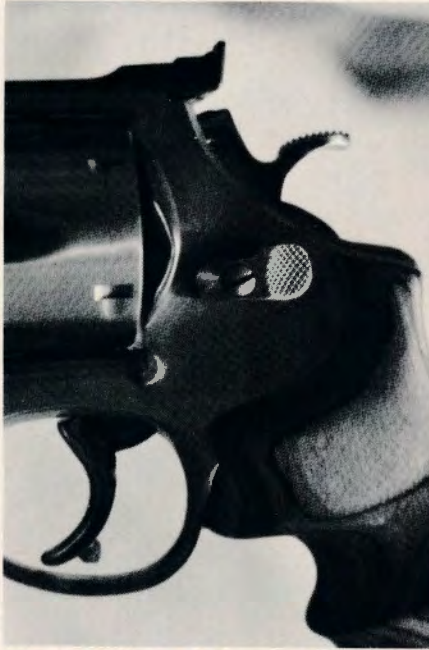
Ayoob's Cannon Custom 4x.44 features a smoothed cylinder release button, polished and shaped trigger, over-travel stop, Millett rear sights and Hogue Combat Grips. Andy Cannon did the work himself.
