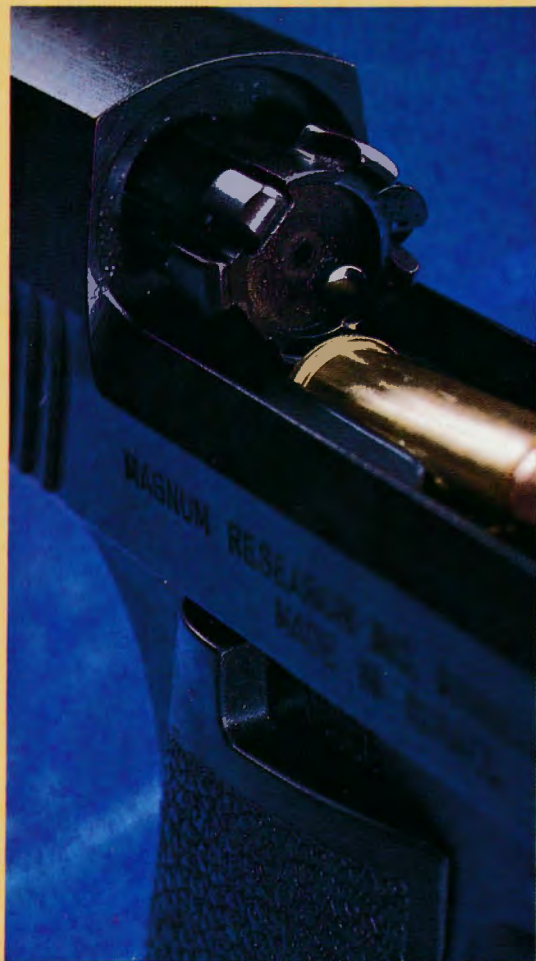
The Desert Eagle uses rotary locking lugs on the bolt, like the M-16. The gas operation helps tame the recoil of the .44 Magnum, as does the weight of the heavy Eagle.
