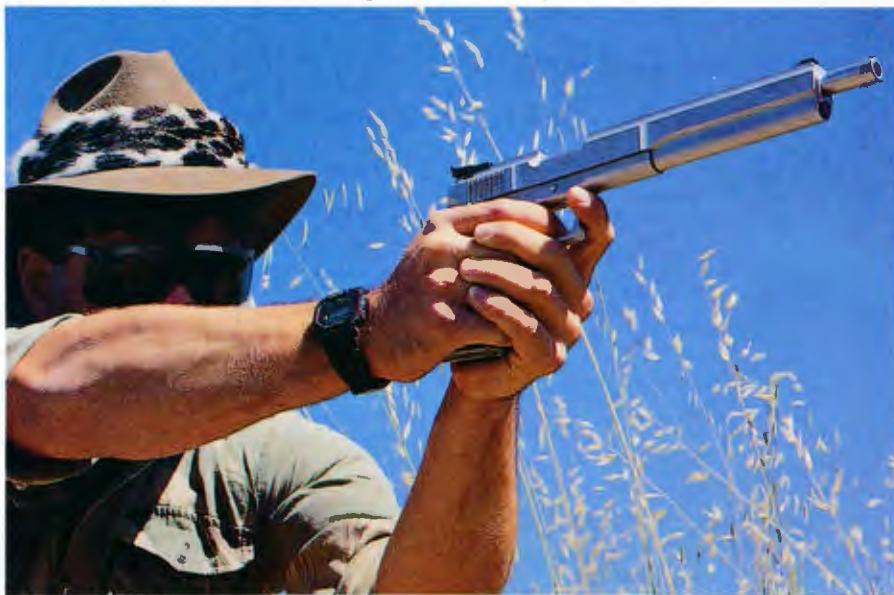
The longslide .45 Magnum Grizzly pistol has a 10-inch barrel and weighs 3.71 pounds unloaded. Yes, it's "muzzle heavy."
