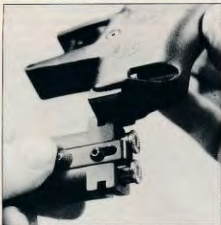
The barrel unit swings outward and upward for loading.
