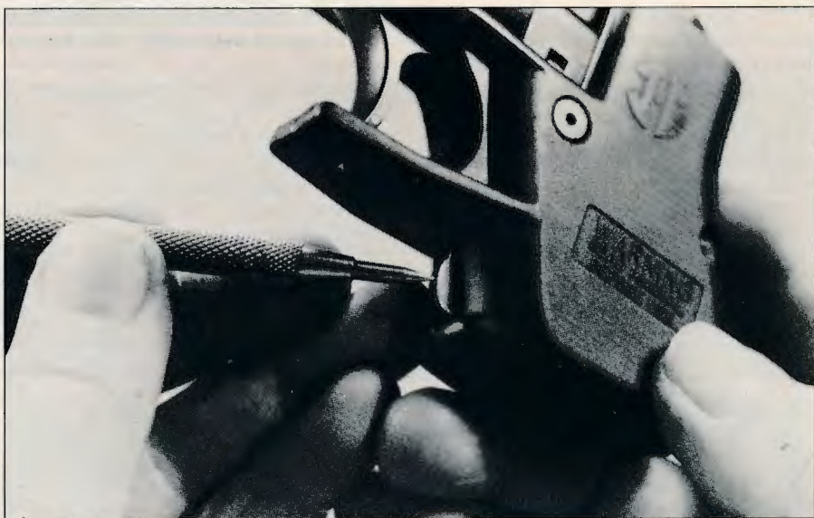
The tool is pointing to the trigger-blocking grip safety pedal. It effectively prevents trigger movement unless the gun is gripped properly.
