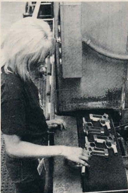
Stainless frames are held on a magnetic conveyor as they are polished by this machine. An S&W worker supervises.
