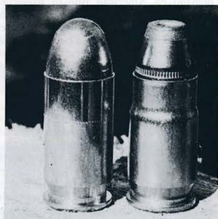
Steps in forming the .357 Bobcat (above): .44 Mag. case is necked to .357, loaded with a 140 gr. JHP and collared. (Right) The .41 Avenger is a .45 ACP case necked to .41 caliber.
