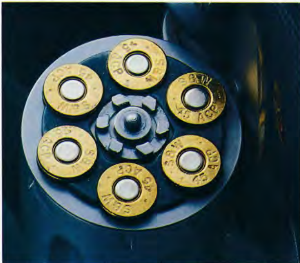
The full moon clip allows rimless .45 ACP cartridges to be extracted by the revolver's star. The clip also provides proper headspacing. Remington's .45 Auto Rim cartridges can be chambered without the clip thanks to the rim that replaces the extractor groove on the ACP case.
