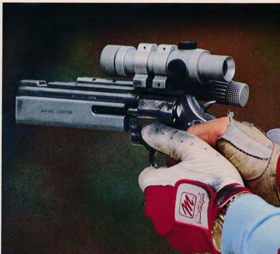
John Pride's quasi-stock Smith 686 has a Jarvis barrel weight underlug, an Aimpoint 2000 sight and an action job. In the esoteric world of Bianchi Cup "race guns," this is pretty plain Jane. Pride won the '88 Cup and always places highly showing that it's the shooter, not the gun, that wins matches.
