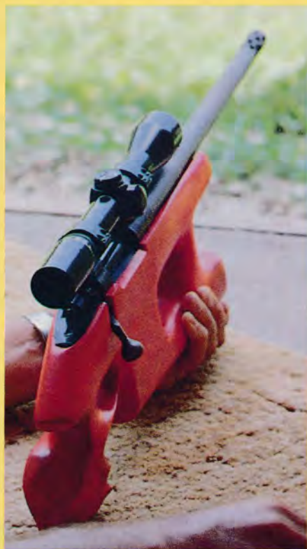
Yes, that's a "handgun" but it's got a rifle action (Sako) and rifle barrel (Douglas) and rifle scope (Tasco).
