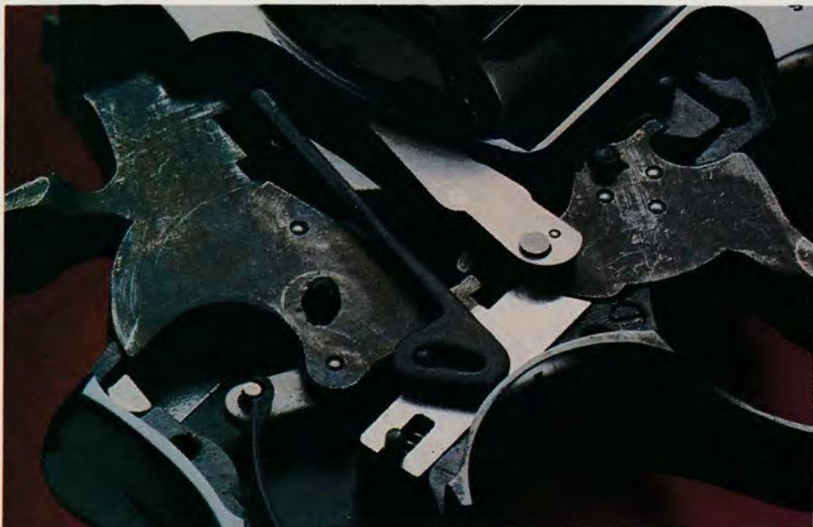
Among the many refinements of Smith & Wesson's classic .22 Masterpiece are a wide target trigger (right), a transfer bar safety to prevent the gun from firing if dropped (above), recessed chambers (above left) and a wide target hammer (top left).
