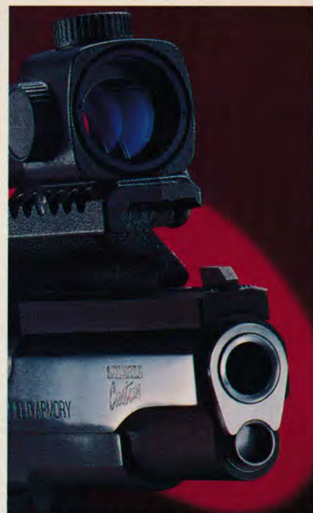
A solid bushing is used on all self-defense custom guns, for reliability.
