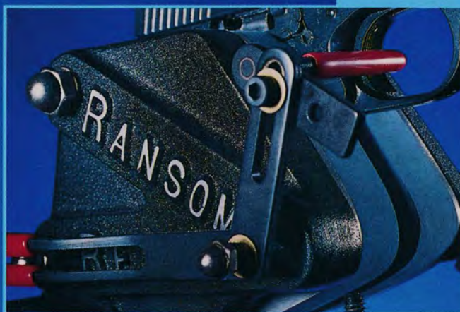
The trigger is activated by an adjustable linkage system that can be set for revolvers and autos alike.
