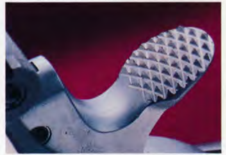
Clockwise from upper left: 1) Today's 629 cylinder does not recess the case heads, a cost-cutting step left over from previous S&W owner Lear Siegler. 2) Mickey Fowler shot the 629 from hunting field-positions. 3) The hammer spur is slimmed down from the honker "target" version. 4) The trigger is smoothed and radiused for improved DA shooting.
