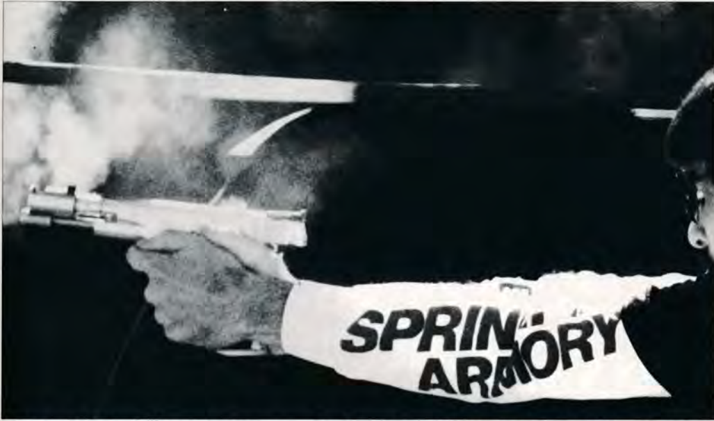
Rick Castelow's .38 Super is puffing smoke like a locomotive even though it's "smokeless" powder. Lead bullets spew smoke worse than jacketed from the grease burning.
