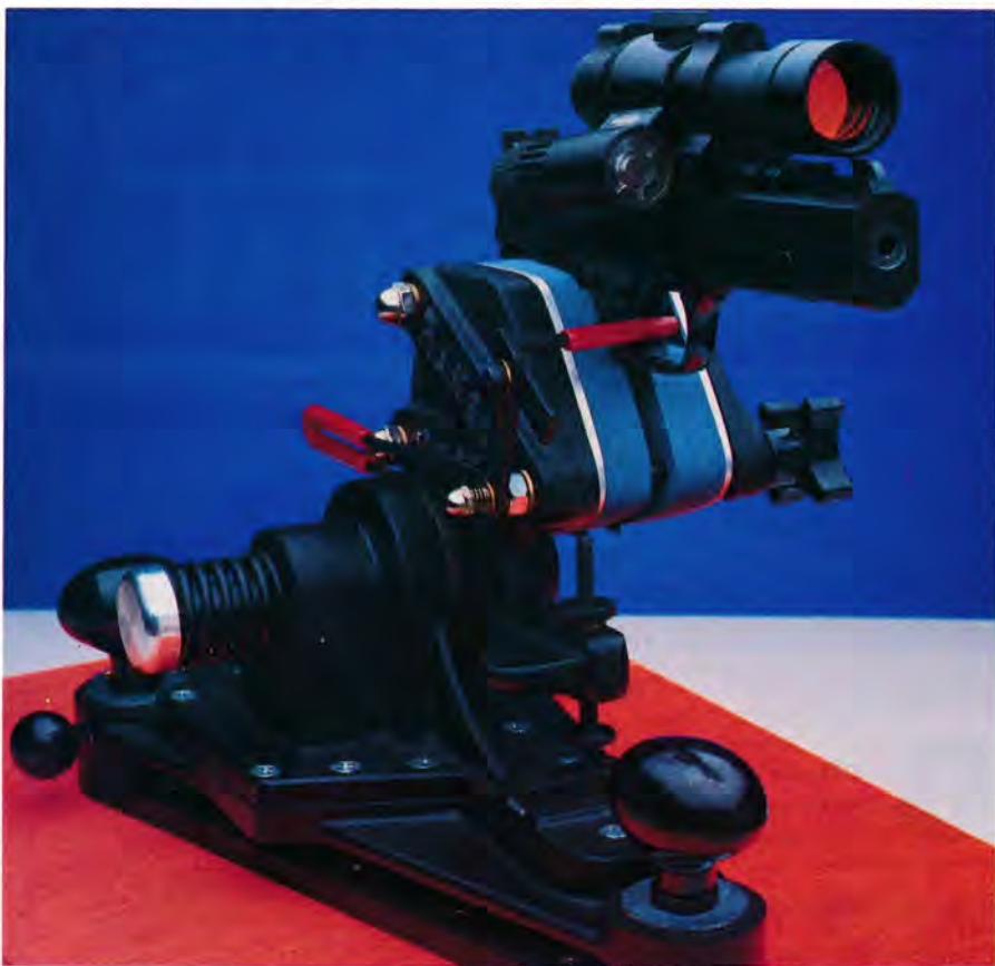
The Ransom Rest allows an auto to feed out of its magazine. You can change mags by tipping the rest upward and accessing the mag well from underneath.
