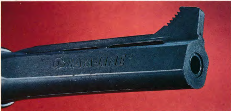
You can see the steel barrel sleeve peeking out from the plastic outer shroud.
