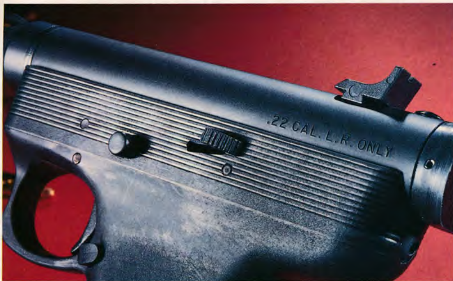
There are three controls on the Exactor: the mag release in the traditional Browning location on the grip; the slide release button just above the trigger guard; and the sliding safety, which is easy to operate.
