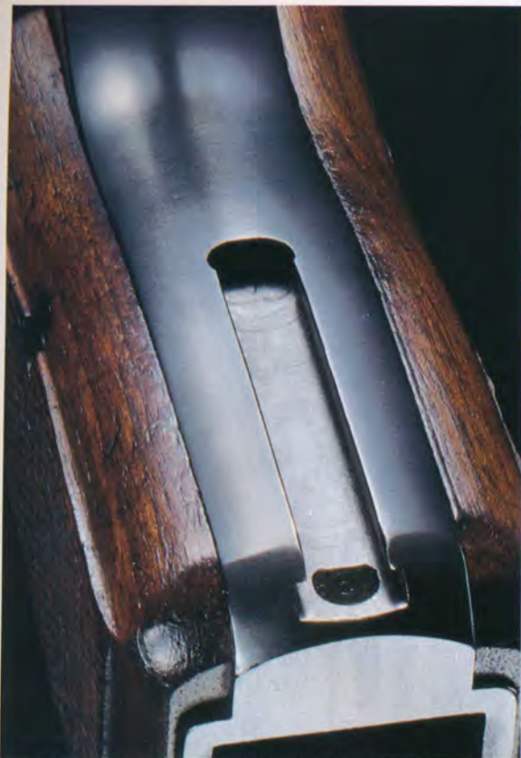
Early Hi-Powers were fitted with detachable shoulder stocks that locked into a slot in the backstrap. Right, the four-digit serial number shows it was made in 1935, the year of introduction.
