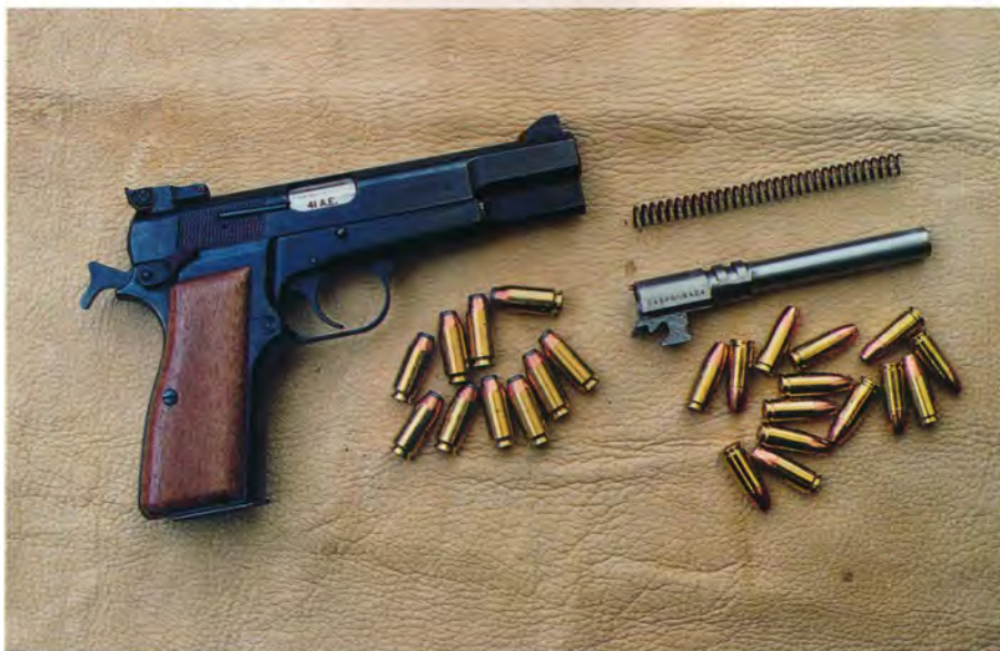
While the .41 AE has been eclipsed by the .40 S&W, the rebated 9mm-size rim of the .41 makes it suitable for upgrading 9mm pistols to a medium-bore.
